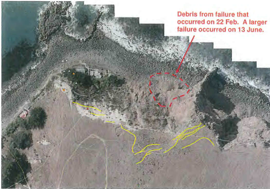
Map of tension cracks (yellow lines) on slopes above Boulder Bay. Tension cracks were originally mapped in late October 2011. Aerial photo is from late February 2011.
